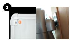
Insert the panel in the clips (C) previously fixed to the wall, using the two hooks (G) located on the sides of the panel (on the back).
